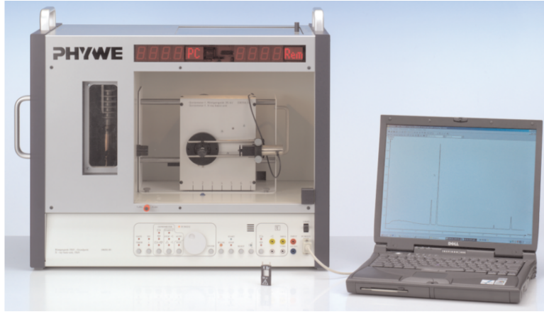
Figure 4: PHYWE 09058.99 X-ray diffraction system showing the main unit (left) with X-ray source, sample holder, and detector, connected to the control computer (right).
